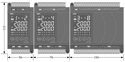
The maximum height of the controller (including the terminal) is 112mm; The width of the controller is 56mm, 76mm and 116mm. The depth of the controller is 78mm.
