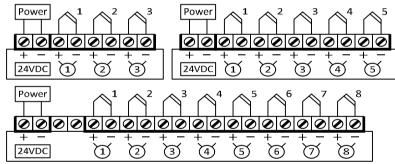
2) Power supply and thermistor signal input
