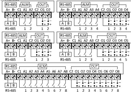
2) Rs-485 communication and relay control output (used to drive ac contactor, etc.)
